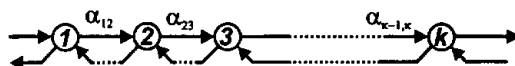
Figure 6. Sequence of irreversible reactions, which at each stage have a reverse pathway, leading from product to the predecessor.
